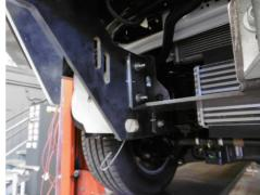
Note: Photo has front of winch frame removed to show bolts in chassis mount
